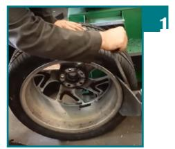
Release air from the tyre by removing the valve. Place the wheel on the tyre changing machine and break both beads. Ensure the sensor is on the opposite side of the breaking bead.
