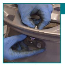
Locate the sensor body on to the other end of the valve stem. Hand-tighten to secure and then tighten the connecting screw to 2.2Nm.
