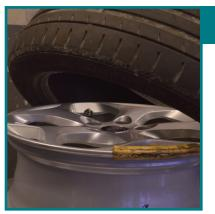
Place the wheel on the turntable and demount the tyre. The sensor can then be removed.
